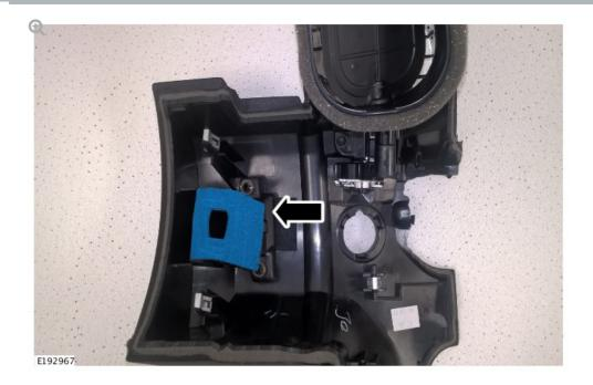
Install the interior temperature sensor insulator foam to the duct behind the sensor grille.
