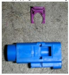
Then on the other side of the Fakra connection there is a plastic leg that locks the cable in to the plug using a small screw driver gently lever the leg up whilst pulling on the cable to release the cable from the plug.
