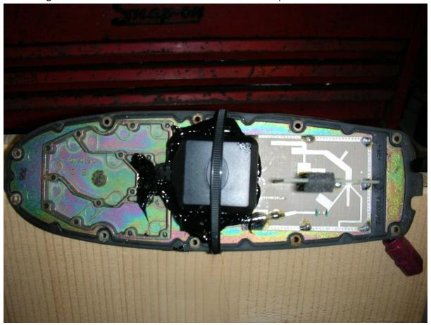
Let the silicon dry and just trim off any excess that's not needed, then you can fit the aerial cover back on and tighten all the 10 T8 screws.
