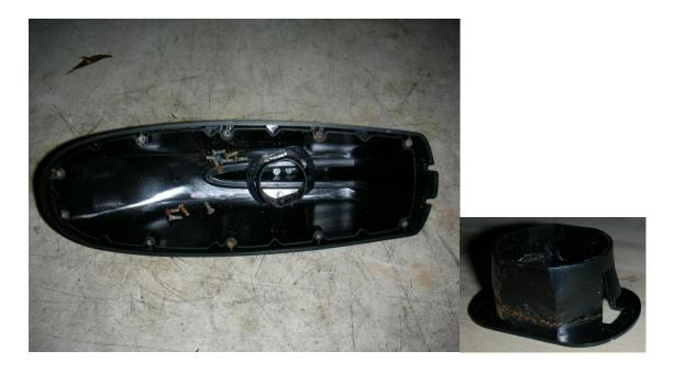
Now you need to remove the 4 T8 screws that hold the GPS aerial to the baseplate and cut the wire see picture below
