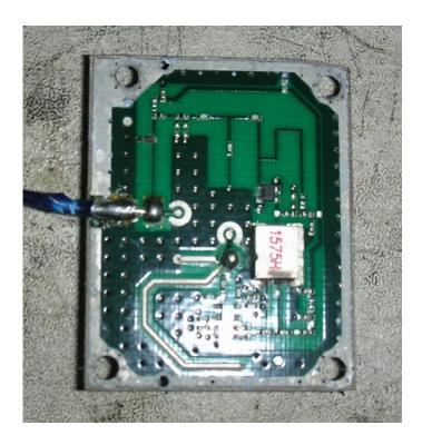
Now with your new cheap GPS aerial you need to remove the blue Fakra Plug on the end, do this by popping out the red locking ring from the plug.
