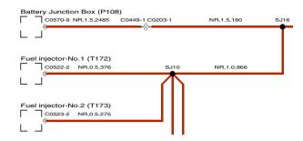
The splices (and where appropriate, the header) circuit pages show the full interconnectivity of components and systems.
