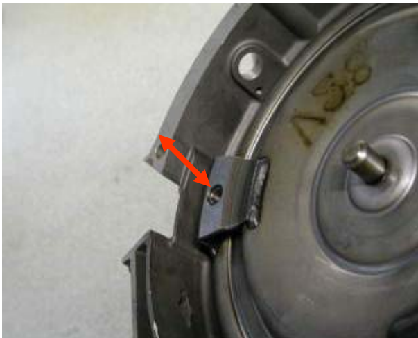
distance from bell housing to torque converter
