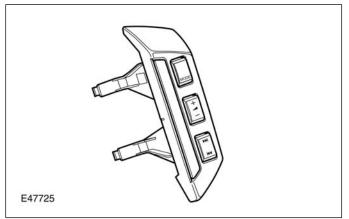
The IHU can be remotely controlled via steering wheel mounted controls. The steering wheel controls are mounted to the right hand side of the steering wheel.
