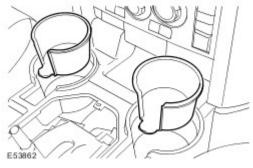
3. Remove the floor console liner.
