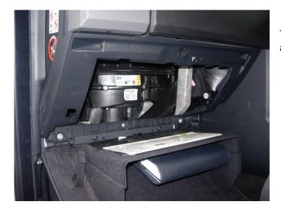
The filer housing is at the top above the fan unit.
