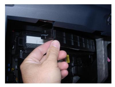
Unclip the front cover from the left hand side and remove.
