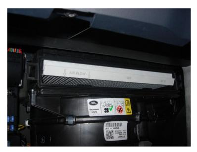
The filer can now be replaced. Take note of the orientation and make sure you insert the new one the correct way around.
