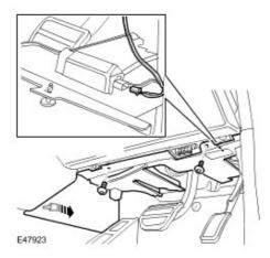
3. Disconnect the steering angle sensor electrical connector.
