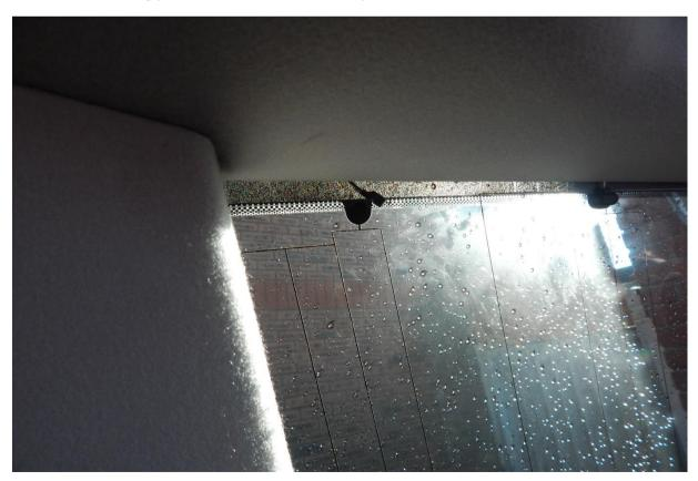
Route the aerial cable from where you will fit the tuner, behind the driver D Pillar to the amps and connect them up
