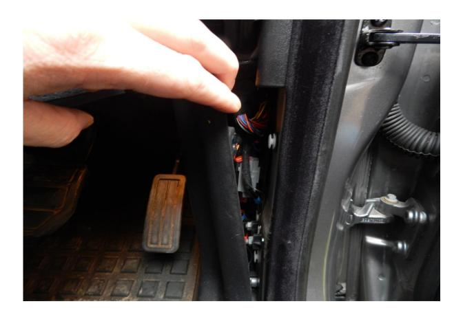
Now Run the Co-Ax cable from here to the rear of the Car (Tucking the Cable under the weather strip, out of the way )
