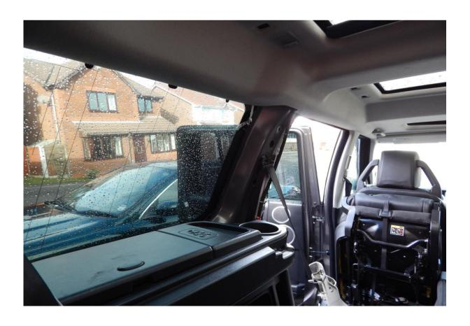
Next Remove Roof lining trim by Removing the two push in type plugs and then the trim releases on clips, disconnect light and then lower the rear of the headlining.
