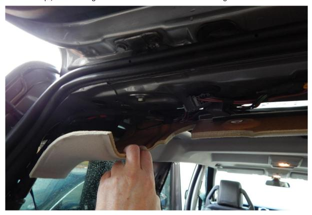
Under the headlining you will have to fit the four amps and route the aerial cable.
