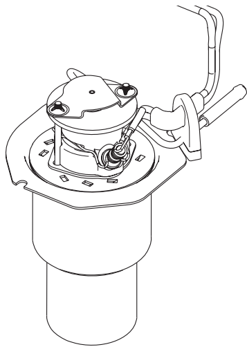
Fig. 208 Diesel burner without fuel preheating
