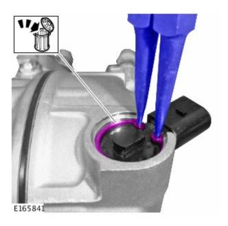
4. CAUTION: Make sure not to damage the housing in the cylinder head.
